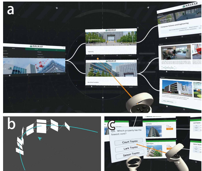
Figure 1: Overview of our system. Our system visualizes all visited web pages and their link structure in a VR space (a). The windows are aligned on a U-shaped curve (b). In the user study, the participants browse a property website (c).
